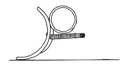
Snow stop will be fixed with the included screws. Place the screw under the tube. Tighten screw to connect both parts.
